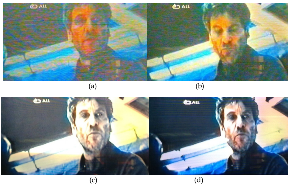
Fig. 14. Video quality of WDM-POF system of (a) 50m, (b) 30m, (c) 20m and (D) 10m of optical transmission line
